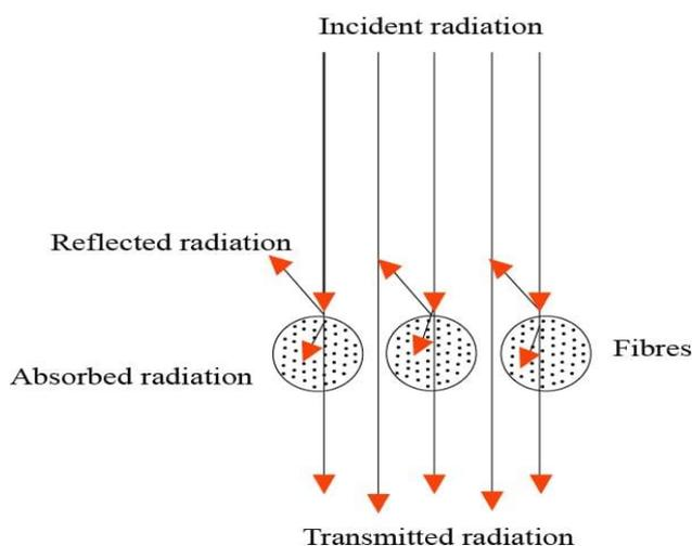
**Figure 16:** radiation in contact with a textile surface
