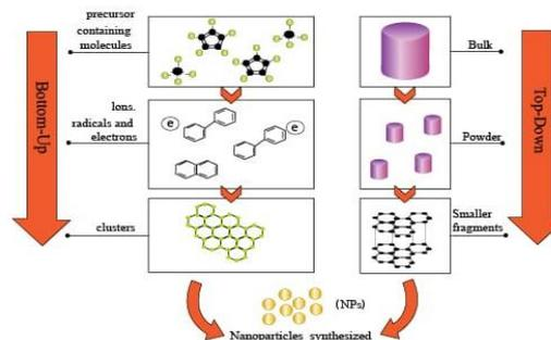
Figure 2: Top-down and bottom-up approaches for the synthesis of NPs
