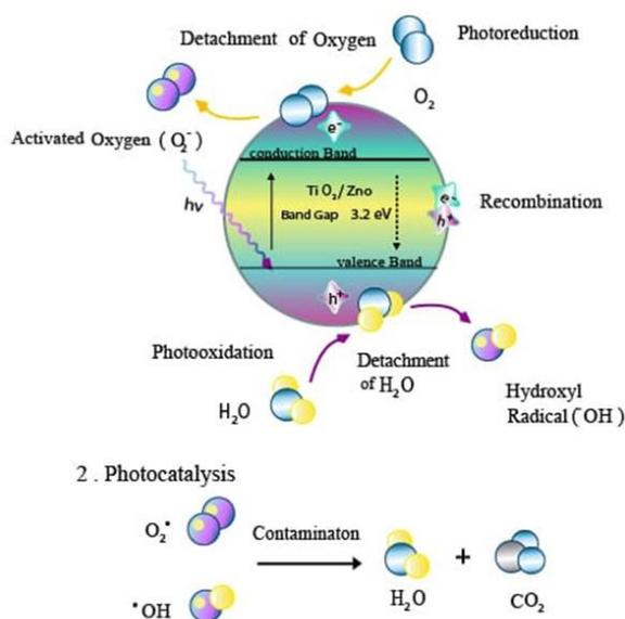
**Figure 18:** photocatalytic activity of  $TiO_2$  nanoparticles
